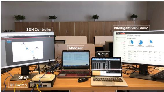
**Figure 3: Demonstrator setup consisting of an SDN Controller, an IntelligentSDS Cloud, an OF Switch, an OF AP, a Victim and an attacker**
