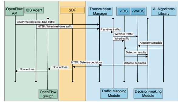
Figure 2: The Sequence Diagram of Auto-defense procedure
