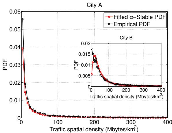
Fig. 4. The results after fitting traffic spatial density to  $\alpha$ -Stable distribution in City A and City B, when sampling window size equals  $3 \times 3$  km<sup>2</sup>.
