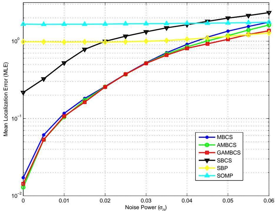
Fig. 7. Localization performance as a function of increasing noise power ( $\sigma_0$ ) for MBCS, AMBCS, GAMBCS, SBCS, SBP and SOMP when there exist 10 MDs and 60 measurements are sampled at the CU side.
