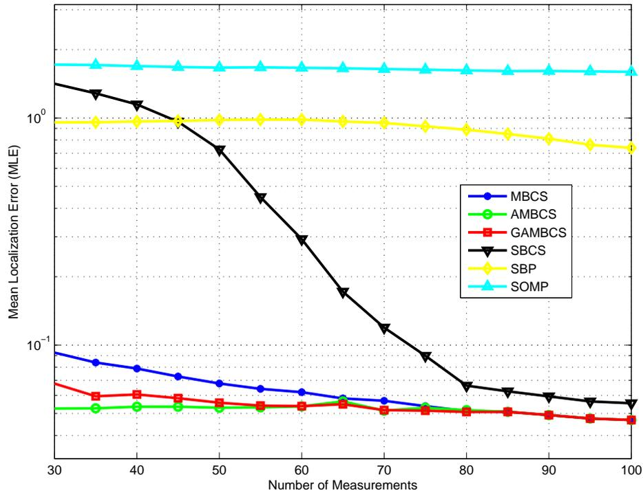
Fig. 3. Localization performance versus varying number of measurements for the algorithms when there exist 10 MDs and noise power  $\sigma_0 = 0.005$ . For AMBCS and GAMBCS, the initial number of measurements is varying and the NEB is set to be 70.
