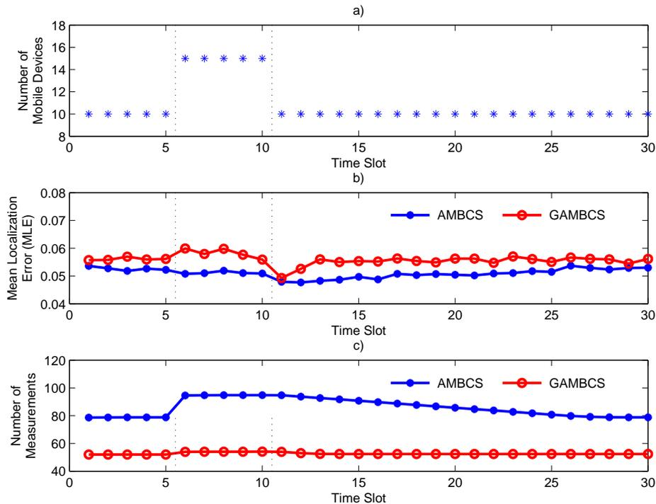
Fig. 5. Localization performance as a function of varying number of mobile devices (MDs) for AMBCS and GAMBCS when initial number of measurements is set to be 50, NEB is set to be 70 and noise power  $\sigma_0 = 0.005$ .
