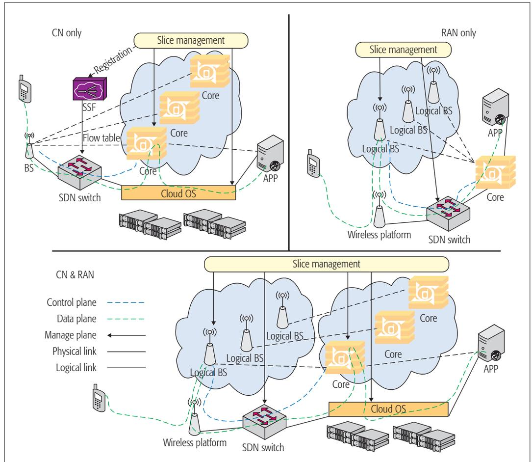
Figure 1. The architecture of three forms of NS.
