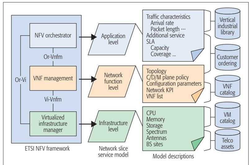
Figure 2. The proposed service models of network slicing.
