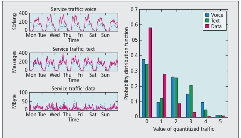
**Figure 1.** (Left) Two typical cells' traffic in one week with different entropies. The random entropies of voice, text and data for the cell in the red solid line are 2.4034, 2.1177, and 2.0415 while the counterparts for the cell in the blue dash line are 2.1834, 2.1733, and 1.5472. (Right) The corresponding probability distribution function with respect to the traffic in the cell in the blue dash line on the left side.
